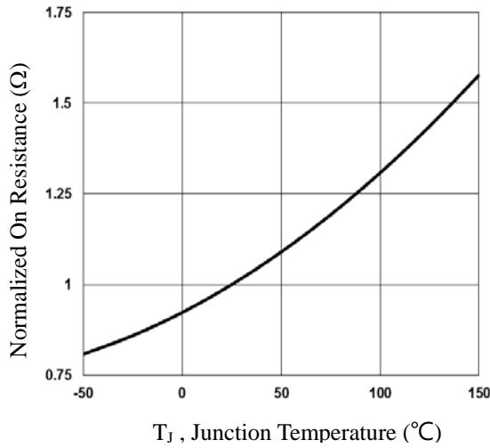
Fig.2 Normalized RDS<sub>ON</sub> vs.  $T_j$
