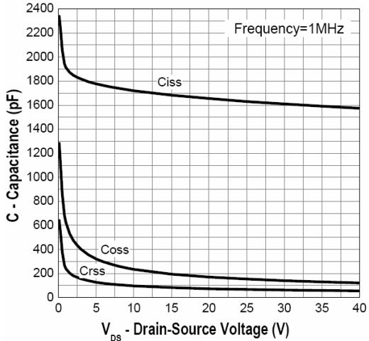
Fig.8 Capacitance Characteristics
