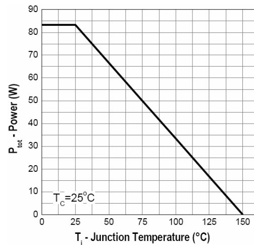
Fig.10 Power Dissipation
